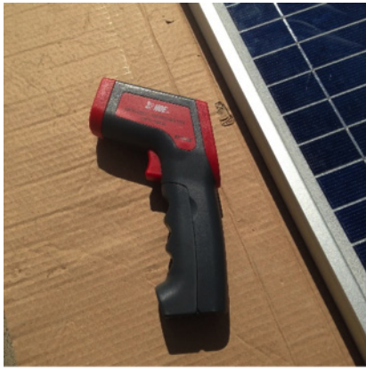
Figure 9. A non-contact thermometer is simple to use to record the surface temperature of the solar cell when taken from the back side (white) of the module. Source: Author
