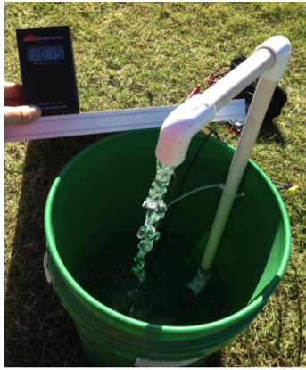
Figure 7. The sunlight irradiance level is read with the pyranometer. The meter rests on the frame of the solar PV module and pointed toward the sun. As the level of the sunlight intensity approaches 1,000 W/m 2 , the solar PV module is producing at the manufacturers rated power. Source: Author
