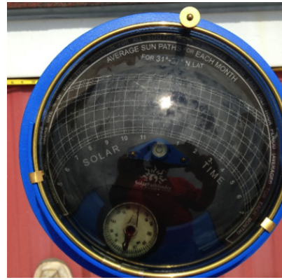
Figure 10. The Solar Pathfinder™ is a site assessment tool used to help the PV system installer determine the suitability of a site by examining the amount of potential shading cast on the location from nearby trees, buildings, utility poles, lines, chimneys, and vent stacks. Source: Author
