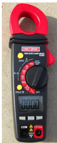
Figure 3. Example of an AC/DC Clamp-On Meter. This model shows no leads connected to the meter. This style meter may be used to measure voltage and amperage. Source: Author
