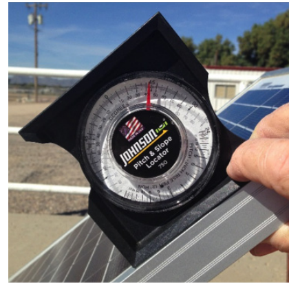
Figure 8. The angle finder is an expensive tool used to check the tilt angle of the module. The finder is set on the frame of the module and the angle in degrees can be read on tool. Source: Author
