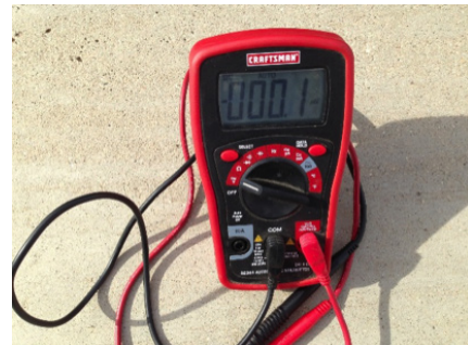
Figure 1. A digital multimeter with leads connected. This tool can be used to measure circuit voltage, continuity, and resistance. Source: Author
