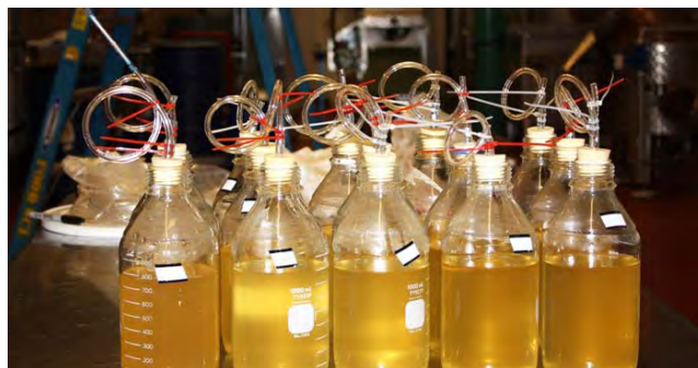
Vessels and test apparatus used to determine elemental sulfur from spray applications in fermenting wines and juice. One goal of the project is to find out how long before harvest sulfur applications need to be stopped to avoid impacts during fermentation.
