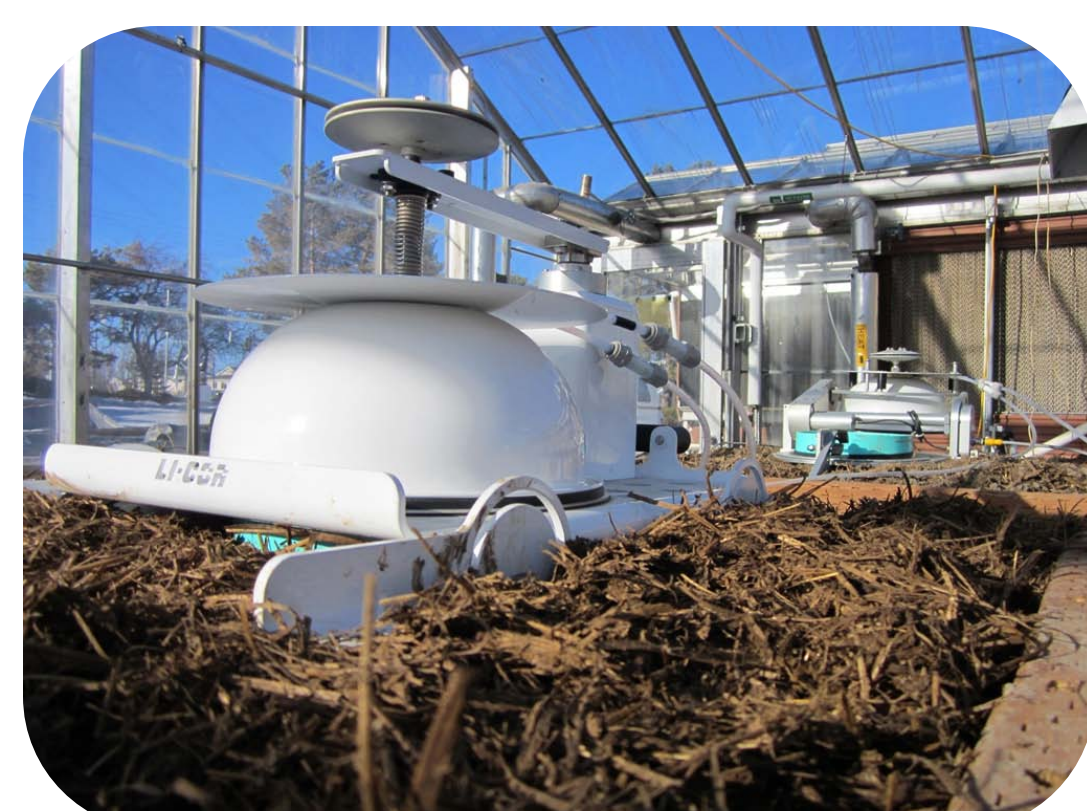
Closed dynamic chambers (CDC) coupled with a multiplexed Fourier Transformed Infrared (FTIR) spectroscopy gas analyzer provided gas flux estimates.
